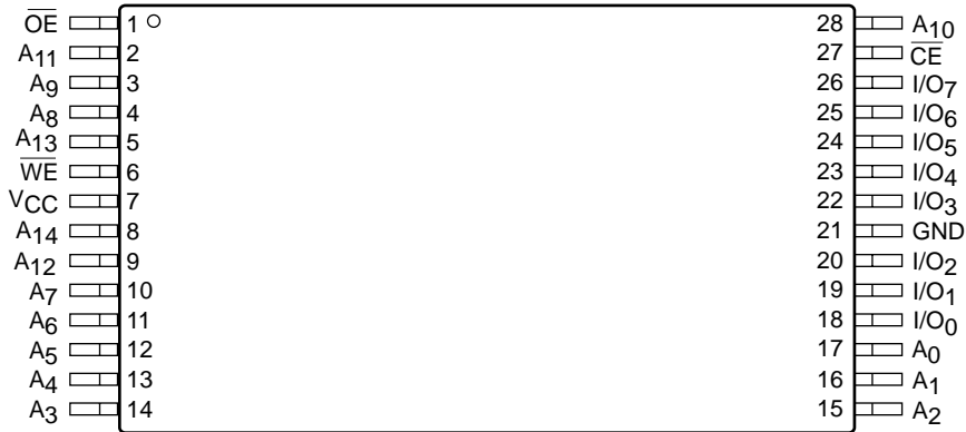
TSOP Top View (8mm X 13.4mm) (T13)
